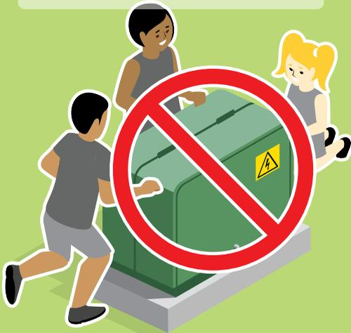
Keep areas surrounding the pad-mounted transformer clear so that workers can safely maintain transformers as needed. Keep shrubs and structures at least 10 feet away from the transformer doors and 4 feet away from the sides.
